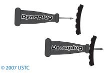
6. Pull tool from hole. Plug will remain in hole. For most punctures from nails and screws, one plug is sufficient.
